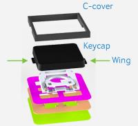
Two wings on each sides of keycap to prevent the key is pulled by restless fingers. When the keycap is pulled, the wings will be blocked by the C-cover.
